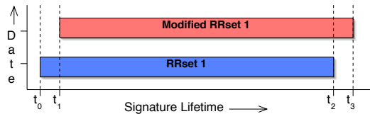
Figure 2: If data changes, such as in “Modified RRset 1”, then the old RRset 1 will still be verified by the zone’s keys (even though the data is no longer valid).
