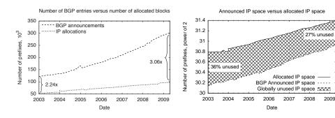
**Fig. 1.** Number of BGP entries compared to number of allocated IP blocks
