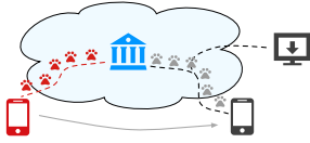
Fig. 3. Conceptual illustration of tracing-based solutions: consumer’s interests are forwarded toward the RV, they may meet the MP-trace along the way and move toward the MP without going through the RV.
