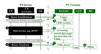
Figure 2: Charging procedures for a data service flow.
