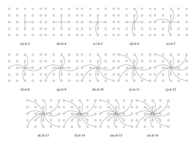
Figure 2. Constructing links for a node with degree(d) from 3 to 16
