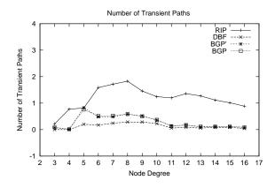
Figure 8. Extra Forwarding Paths Traversed by Packets
