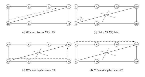
Figure 1. Packet Could still Be Delivered during Convergence
